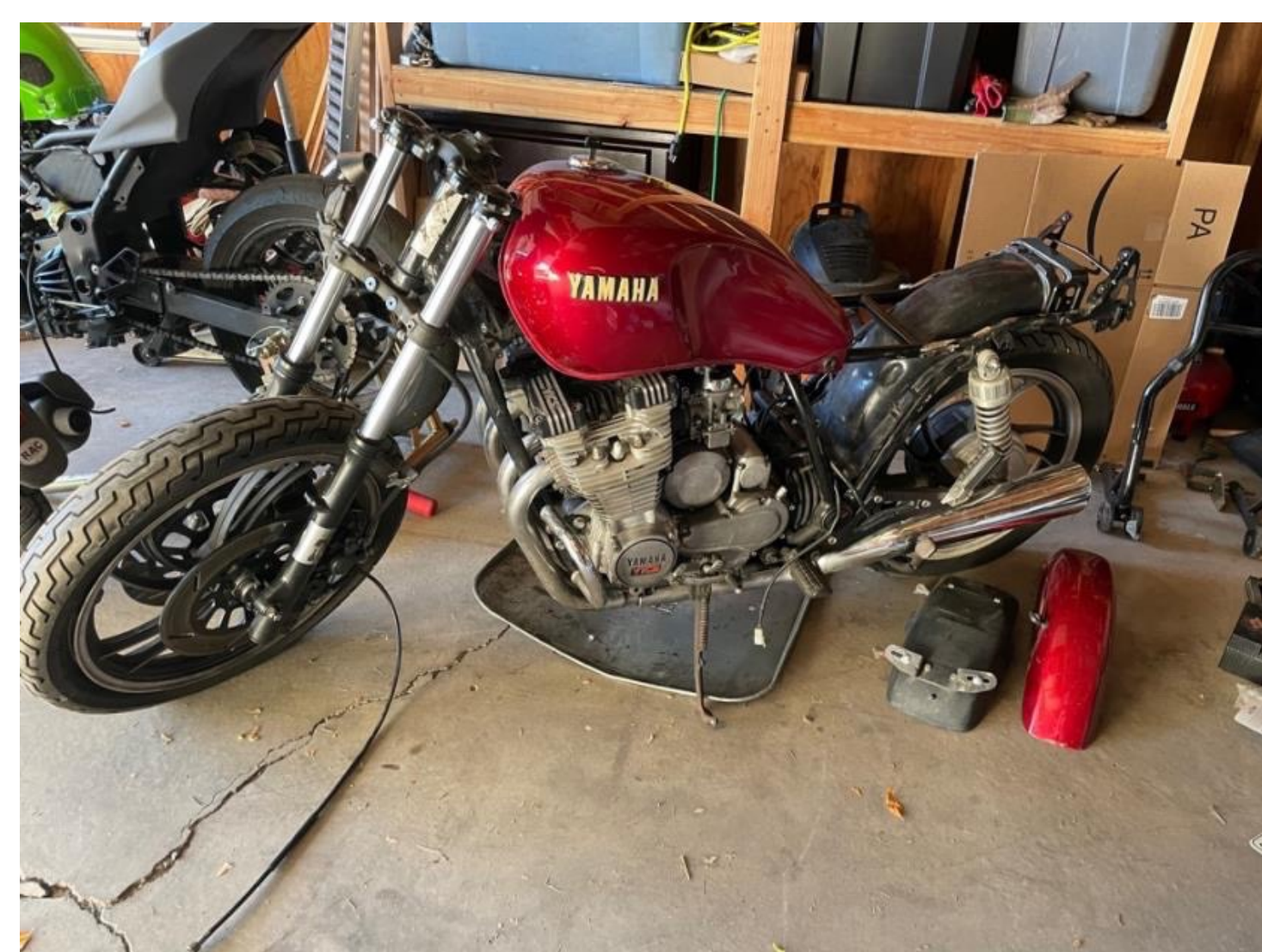
Fig 4: Initial fuel tank test fitting
