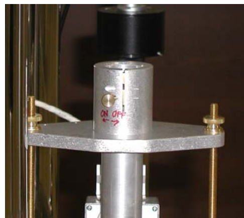
Figure 5: Sample Catcher for Emergency Eject System
