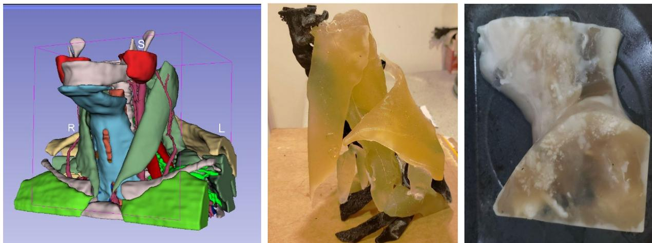
*Figure 1: Creation of an ultrasound phantom of the interscalene space. The 3D model created from patient CT scan (A), assembly of the ballistic gelatin muscular structures (B), and the completed phantom (C).*
