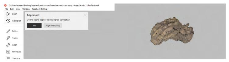
Once auto align has done its job, rotate around the model a few times to make sure that they are sitting atop each other properly. If they are not, click the 'Align manually' tool to give the program a helping hand in making sure the scans are properly aligned.
