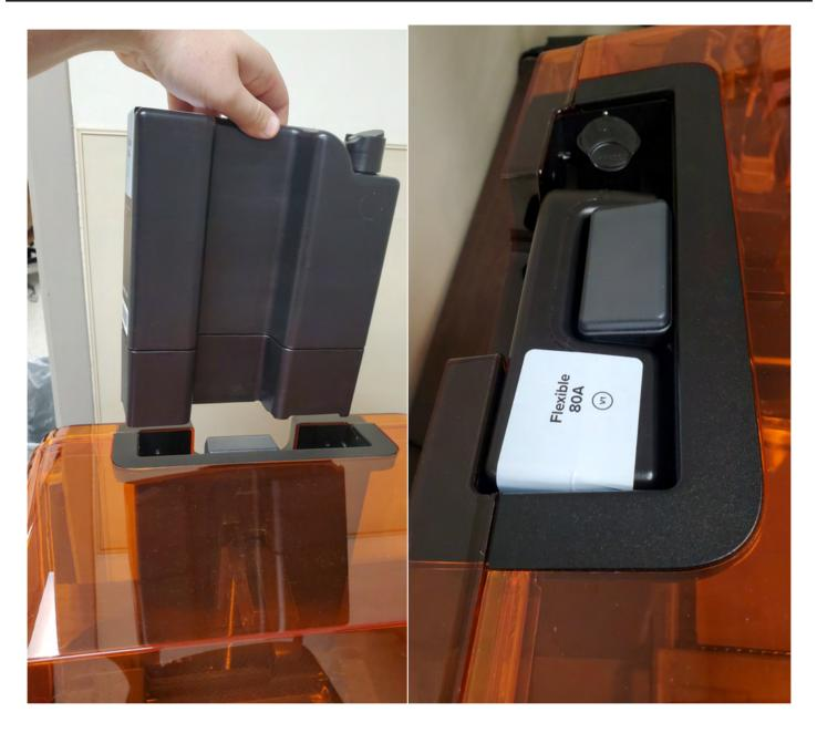
The second part of changing the resin has to do with the tank located on the back of the printer. Each tank can be cleanly and safely lifted from the back of the machine and placed away in storage. When not printing and when storing the tank, make sure that the pour nozzle located on the top of the tank is closed. When printing an object, press down on the tab to open the pour nozzle to allow the resin to flow into the printer properly.
