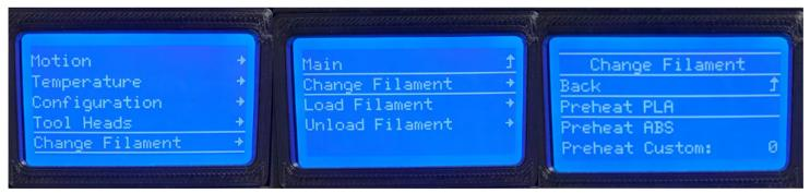
Scroll down to 'Change Filament'. Press in to select.
