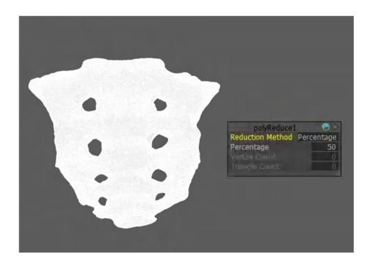
Once the computer has finished calculating the lines of the model will turn white instead of green. Alongside that, an information box will pop up informing you of how the model was reduced and by what percentage. Unless you're aiming for a specific polycount, reducing by percentage is the most reliable method. If you need to reduce the polycount further you can either increase the percentage that the polycount is reduced, or put the model through another Reduce cycle.
