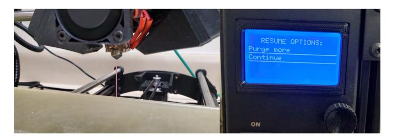
If you inserted the filament correctly, you should see a steady stream of filament coming from the nozzle as the printer purges the old filament to be replaced by the new. If the filament is coming out the correct color, you can click continue on the screen. If the filament isn't coming out of the nozzle or if it is coming out the wrong color, click on 'Purge More' until the correct color is flowing out of the nozzle below.
